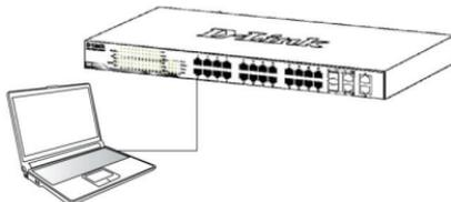
Figure 6. Connected Ethernet cable
