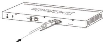
Figure 2-2. Connect the power cord to the Switch
