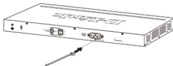
Figure 2-1. Insert Tie Wrap to the Switch
