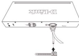
Figure 2-3. Slide the Retainer through the Tie Wrap
