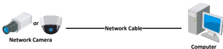
Figure 3-1 Connecting Directly
