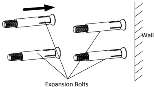
Figure 2-8 Insert Expansion Bolts
