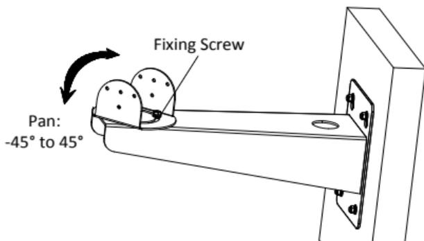
Figure 2-4 Adjust Panning Position
