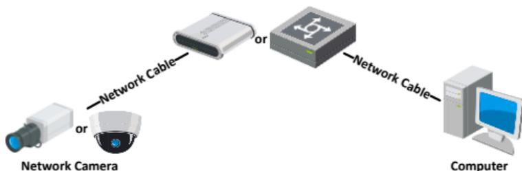
Figure 3-2 Connecting via a Switch or a Router
