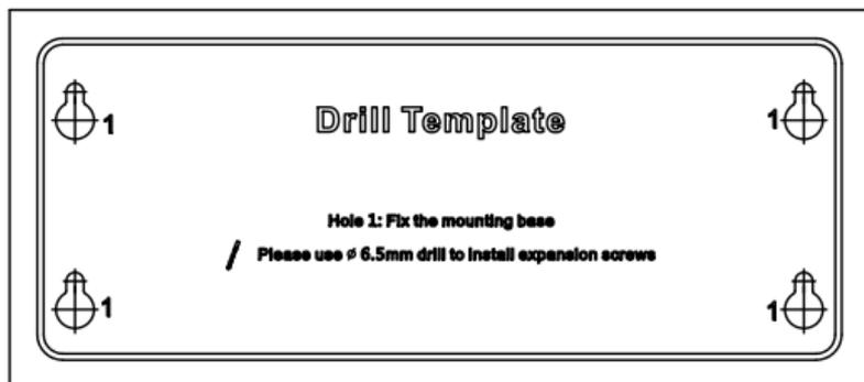
Figure 2-7 Drill Template of Junction Box
