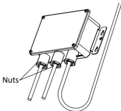
Figure 2-12 Screw the Cover Back
