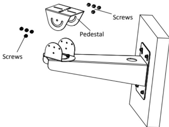
Figure 2-2 Remove the Pedestal
