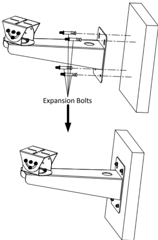
Figure 2-1 Install Wall Mounting Bracket
