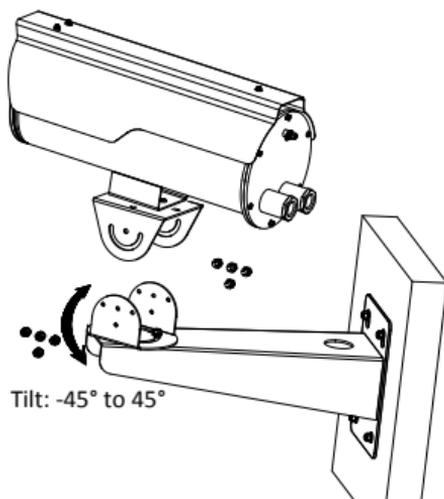
Figure 2-5 Adjust Tilting Position
