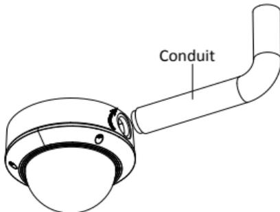
Figure 2-10 Install the Conduit to the Camera
