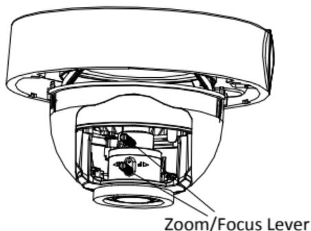
Figure 2-36 Zoom/Focus Lever (Type II Camera)
