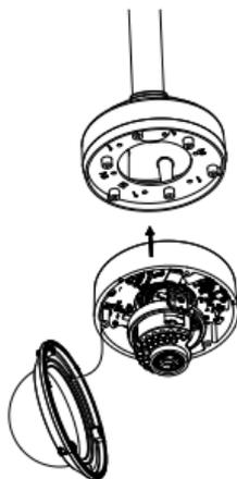
Figure 2-26 Secure the Camera
