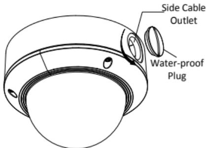
Figure 2-9 Remove the Water-proof Plug
