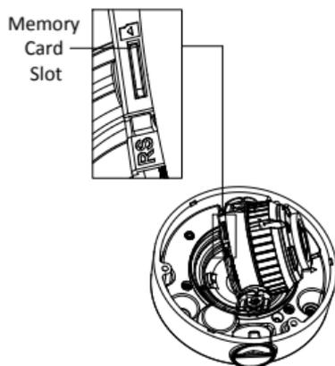
Figure 2-4 Install the Memory Card (Type II Camera)
