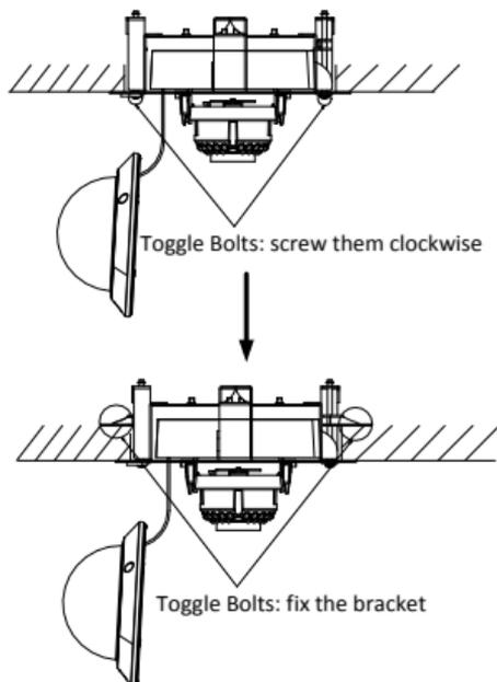
Figure 2-15 Fix the Bracket in Ceiling
