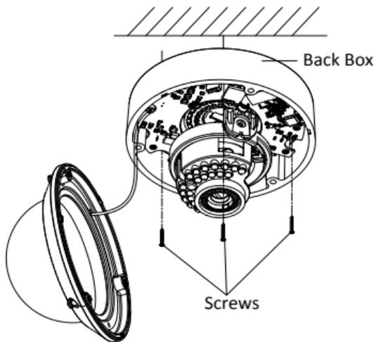
Figure 2-7 Secure the Camera
