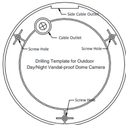
Figure 2-5 The Drill Template (Type I Camera)
