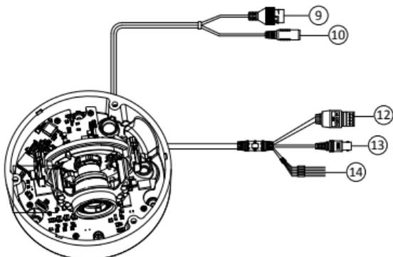
Figure 1-4 Cable Description of Type I Camera (2)
