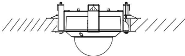
Figure 2-16 Install the Black Liner and the Bubble
