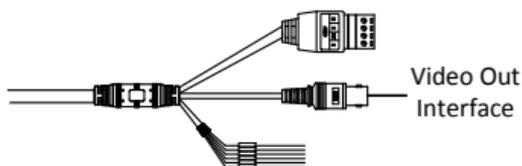
Figure 2-32 Video Out Interface of the Camera
