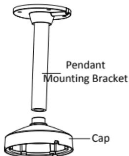
Figure 2-24 Install the Pendant Mounting Bracket
