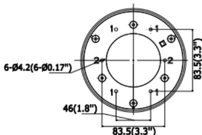
Figure 2-18 Size of the Mounting Base
