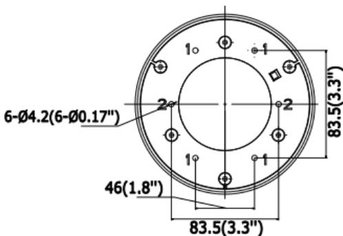
Figure 2-23 Size of the Mounting Base
