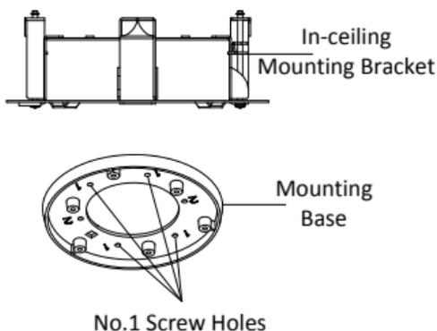
Figure 2-13 Install Mounting Base
