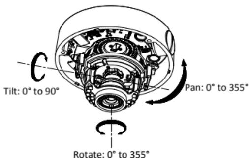
Figure 2-33 3-axis Adjustment (Type I Camera)
