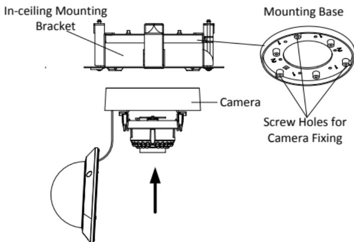
Figure 2-14 Install the Camera to the Mounting Base
