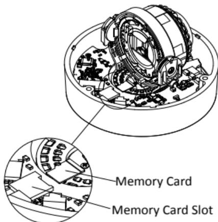
Figure 2-3 Install the Memory Card (Type I Camera)
