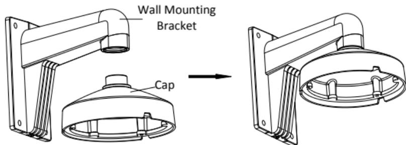
Figure 2-19 Install Wall Mounting Bracket
