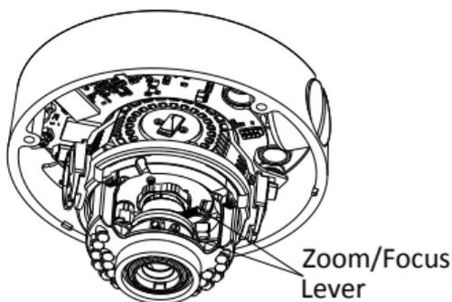
Figure 2-35 Zoom/Focus Lever (Type I Camera)
