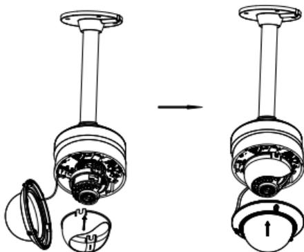
Figure 2-27 Secure Black Liner and Bubble
