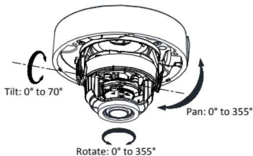
Figure 2-34 3-axis Adjustment (Type II Camera)
