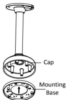
Figure 2-25 Install the Mounting Base
