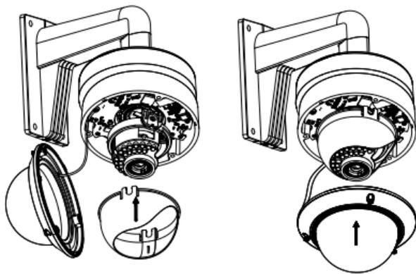
Figure 2-22 Secure Black Liner and Bubble
