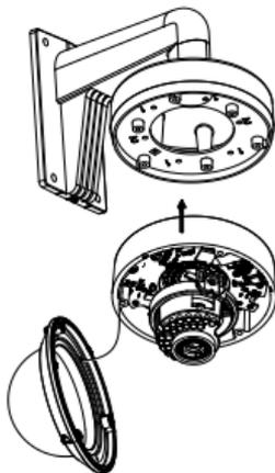
Figure 2-21 Secure the Camera
