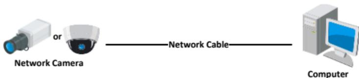
Figure 3-1 Connecting Directly
