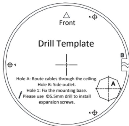
Figure 2-6 The Drill Template (Type II Camera)
