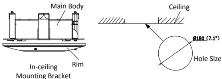
Figure 2-12 Cut a Hole for In-ceiling Mounting
