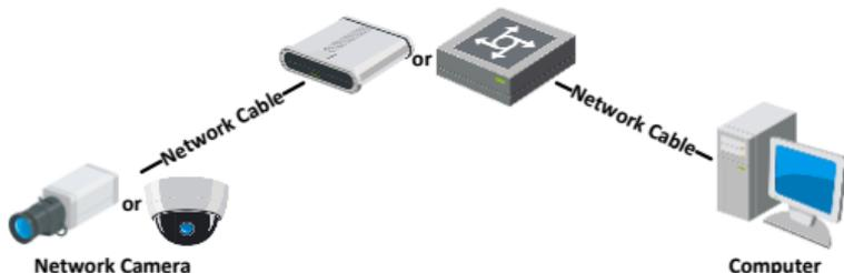
Figure 3-2 Connecting via a Switch or a Router
