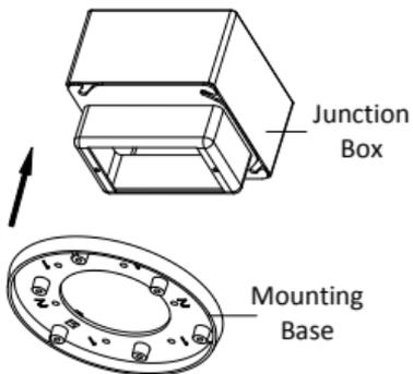
Figure 2-28 Install the Mounting Base
