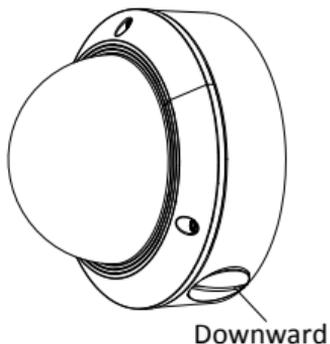
Figure 2-11 Side Outlet Direction
