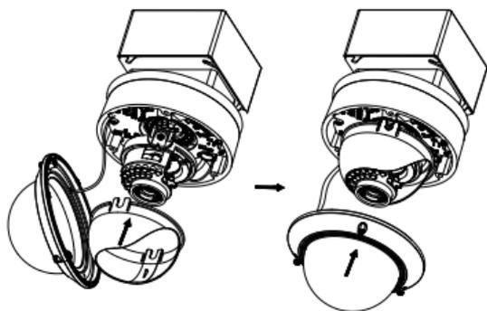
Figure 2-30 Secure the Black Liner and Bubble
