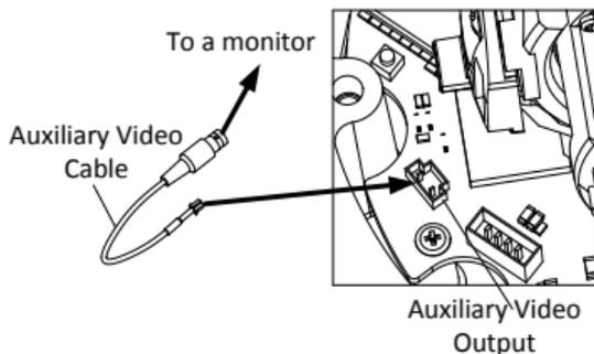
Figure 2-31 Connect Camera to a Monitor
