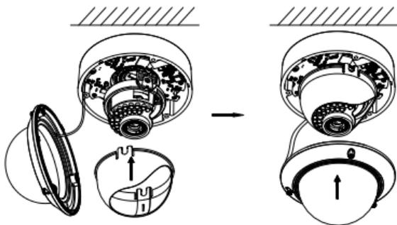
Figure 2-8 Secure Black Liner and Bubble
