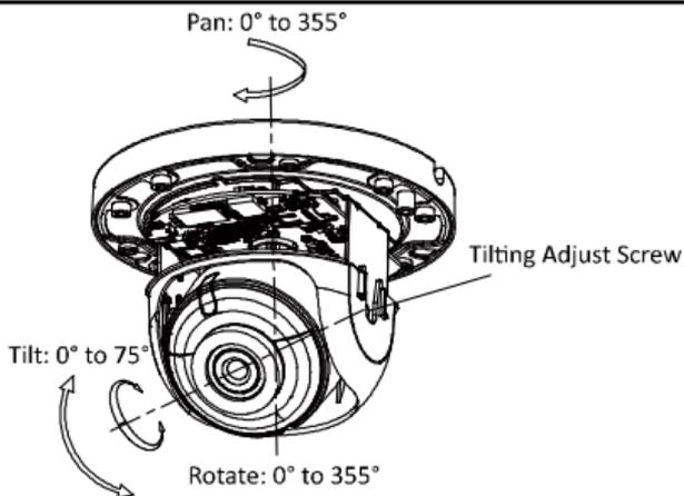
Figure 2-8 Angle Adjustment of Type III Camera
