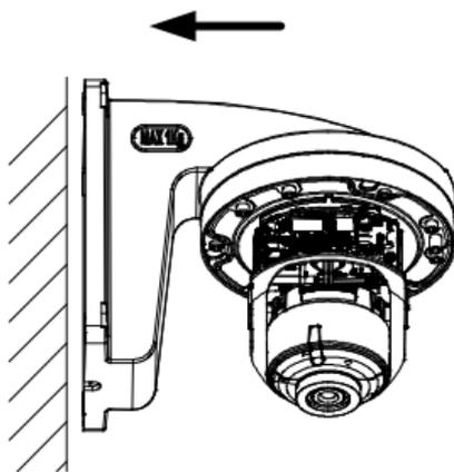
Figure 2-12 Fix the Wall Mounting Bracket to Wall
