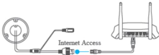
Figure 5-3 Connect a Router
