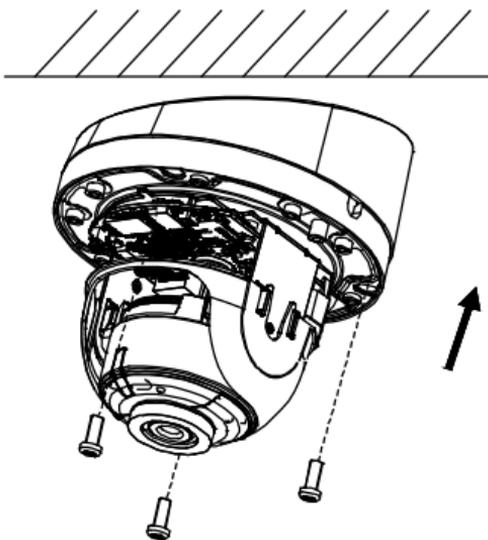
Figure 2-24 Fix the Camera to Wall Mounting Bracket
