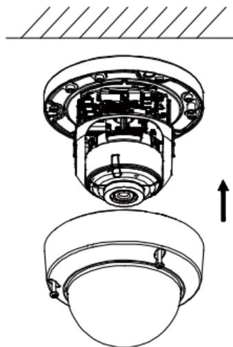
Figure 2-9 Install Bubble
