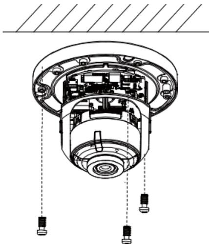
Figure 2-5 Fix the Mounting Base
