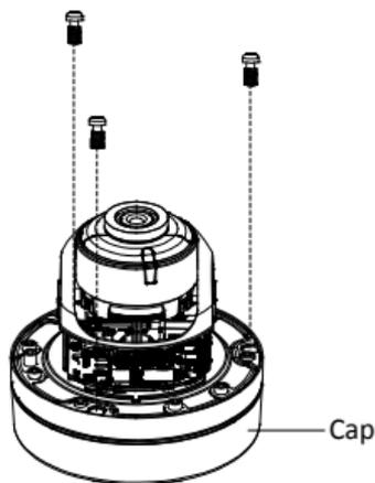
Figure 2-20 Fix the Camera to Cap
