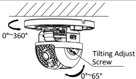
Figure 2-6 Angle Adjustment of Type I Camera
