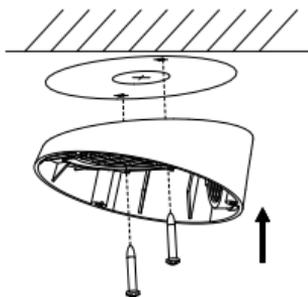
Figure 2-23 Fix Incline Mounting Bracket to Wall
