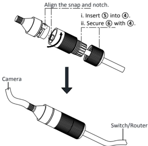
Figure 2-27 Water-proof Accessory Installation
