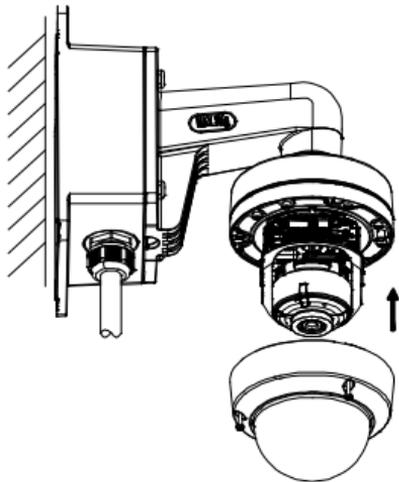
Figure 2-18 Install the Bubble
