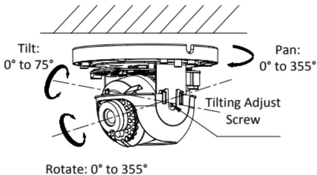
Figure 2-7 Angle Adjustment of Type II Camera
