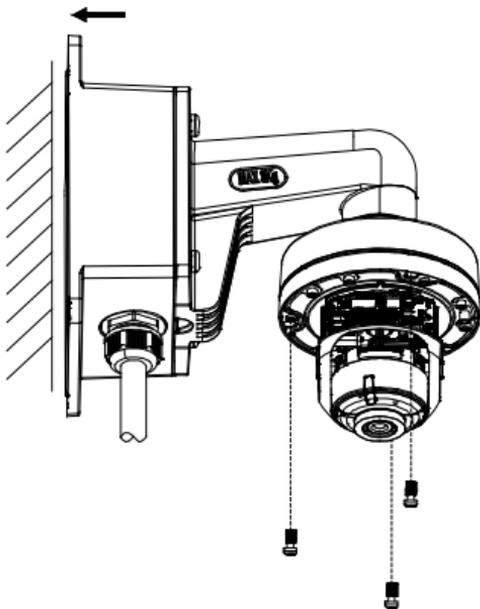
Figure 2-17 Fix the Camera to Wall Mounting Bracket
