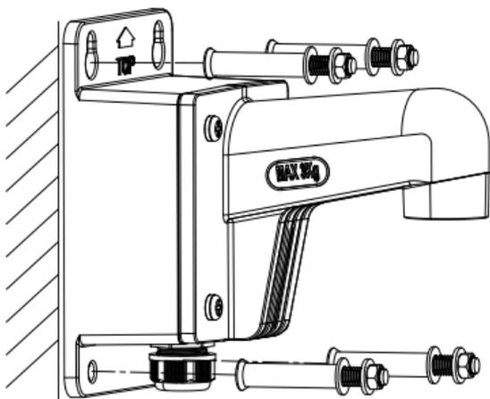
Figure 2-14 Fix the Bracket
