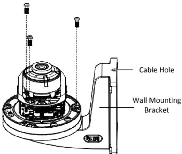
Figure 2-11 Fix the Camera to Wall Mounting Bracket
