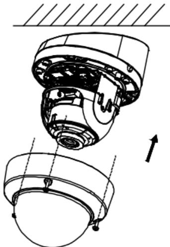
Figure 2-25 Install the Bubble
