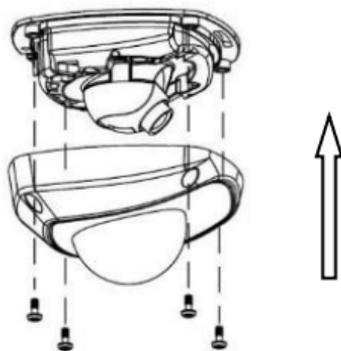
Figure 2-26 Install the Back Box
