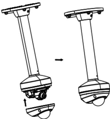
Figure 2-12 Install the Front Cover
