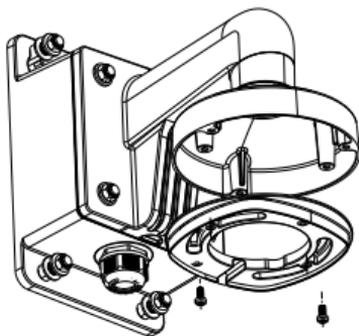
Figure 2-14 Fix the Adapter Plate
