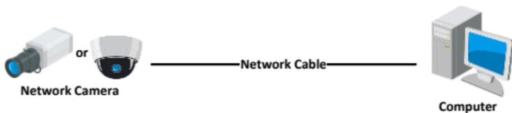
Figure 3-1 Connecting Directly
