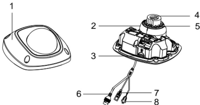
Figure 1-1 Overview of Type I Mini Dome Camera
