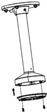
Figure 2-10 Fix the Adapter Plate
