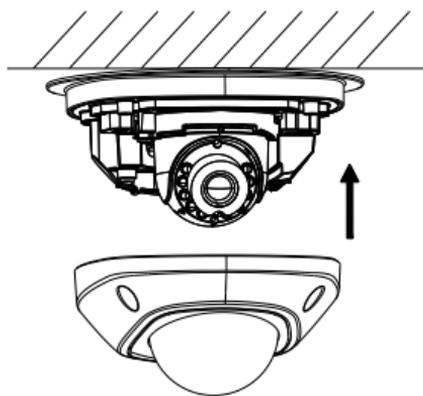
Figure 2-6 Install the Front Cover
