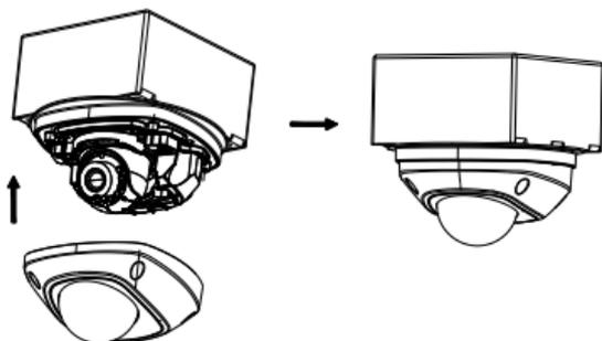
Figure 2-9 Install the Front Cover
