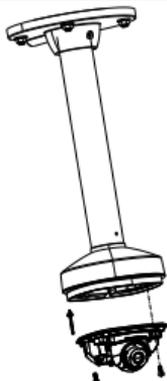
Figure 2-11 Fix the Dome Drive
