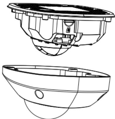
Figure 2-17 Remove the Front Cover
