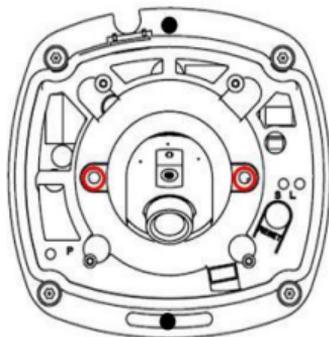
Figure 2-23 Loosen the Lens Set Screws
