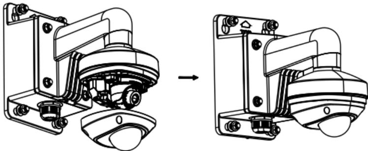
Figure 2-16 Install the Front Cover
