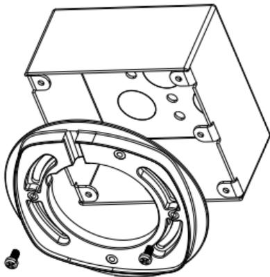
Figure 2-7 Fix the Adapter Plate
