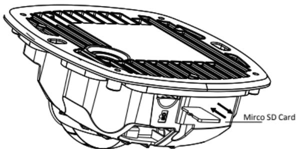
Figure 2-18 Install and Uninstall Micro SD Card
