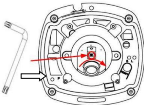
Figure 2-24 Adjust Panning Position
