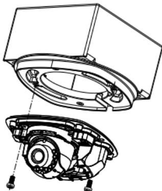
Figure 2-8 Fix the Dome Drive
