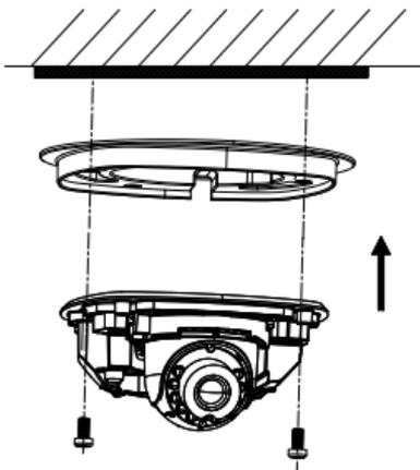
Figure 2-4 Fix the Camera Body
