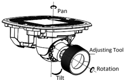
Figure 2-5 3-Axis Adjustment
