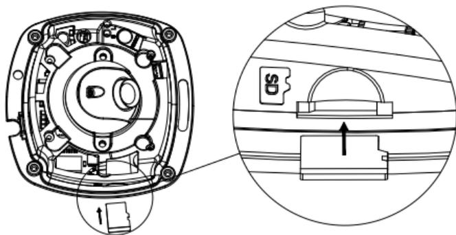
Figure 2-21 Install Micro SD Card
