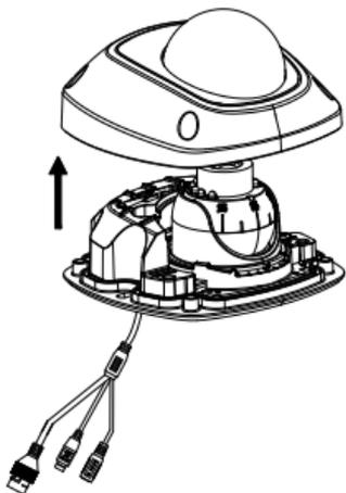
Figure 2-2 Disassemble the Camera
